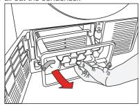
4. Clean the condenser by applying pressurized water with a shower armature and wait until the water drains.
